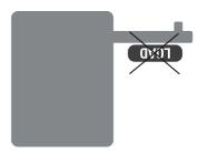
Unwind the power cord. Check that the Crumb Tray is in place and that there is nothing in the oven. Plug power cord into a 220-240Volt AC electrical outlet.
